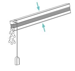
In the case of electrical and crank operated systems, make sure the mechanical parts do not come into contact with the detergent solution or water.
