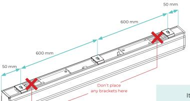
Mount the clips 50 mm from the end of the headrail, and with a distance of max. 600 mm.
