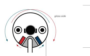
red adjustment bolt = bottom limit blue adjustment bolt = top limit
